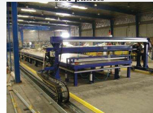
Automated gluing line for big-size panels
