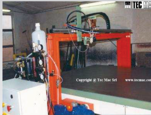
Gluing unit for discontinuous line
