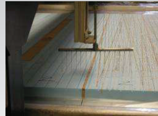
Refrigerated truck gluing
