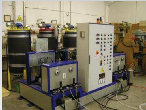
Double gluing unit for continuous line
